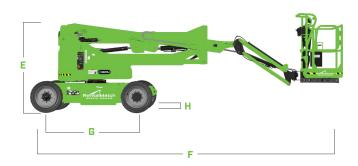
A. Platform Width 30-in / 76-cm B. Platform Length 60-in / 1.52-m 5-ft 9-in / 1.75-m C. Machine Width ■. Tailswing 0-in / 0-cm E. Machine Height 6-ft 7-in / 2.01-m F. Machine Length 21-ft 2-in / 6.45-m G. Wheelbase 6-ft 7-in / 2.01-m 8-in / 20-cm H. Ground Clearance
